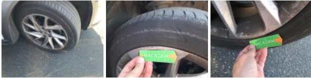
Tyre FR, Out of tolerance, Replace
