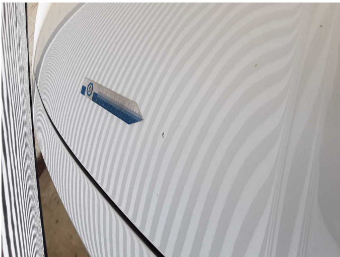
Damage 3: Bonnet: Bonnet - dent(s) - Smooth repair work
