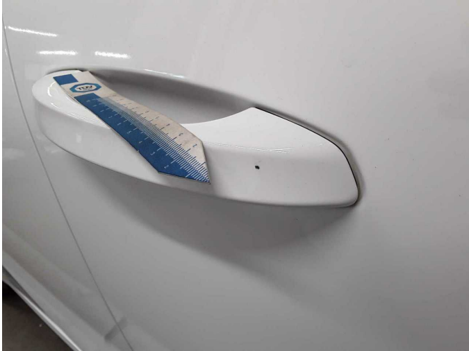
Damage 2: Door - front right side: Door handle - outside - Stone chips - Smart repair
