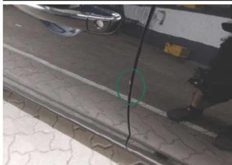
Tür / Vorne Links / Kratzer
