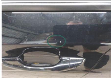
Tür / Vorne Links / Kratzer
