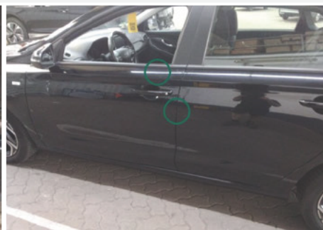
Tür / Vorne Links / Kratzer
