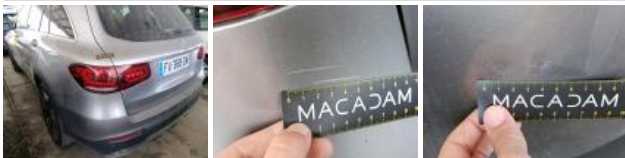
Tailgate / Boot, Dent(s), Repair and paint (complete)
