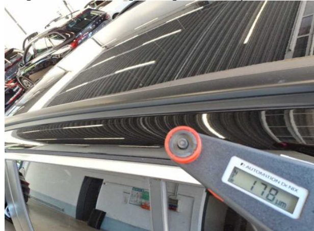
Repainting 1: Roof rail - left side, Roof rail - right side, Mudguard - left side, Mudguard - right side, Side panel - rear
