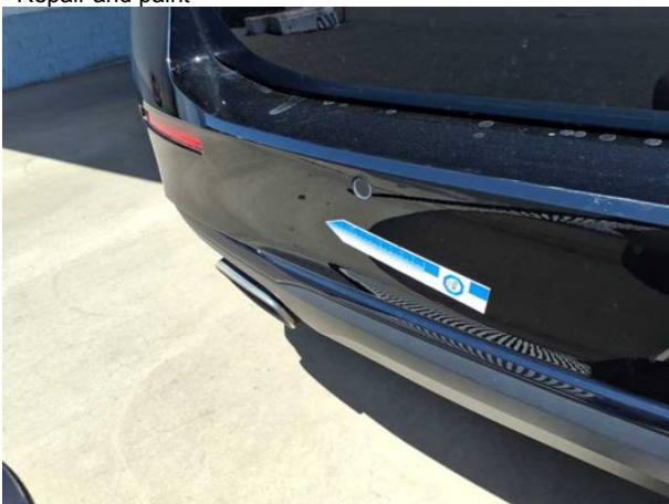
Damage #2: Rear bumper: Rear bumper - Dent / paintcoat damage - Repair and paint
