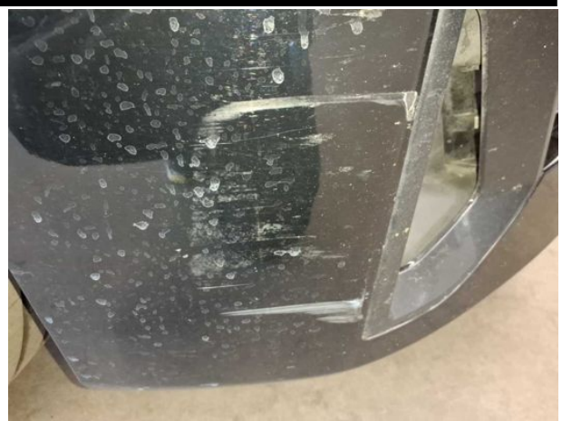
Damage #3: Front bumper: Front bumper - Scratch(es) - Rep... and paint
