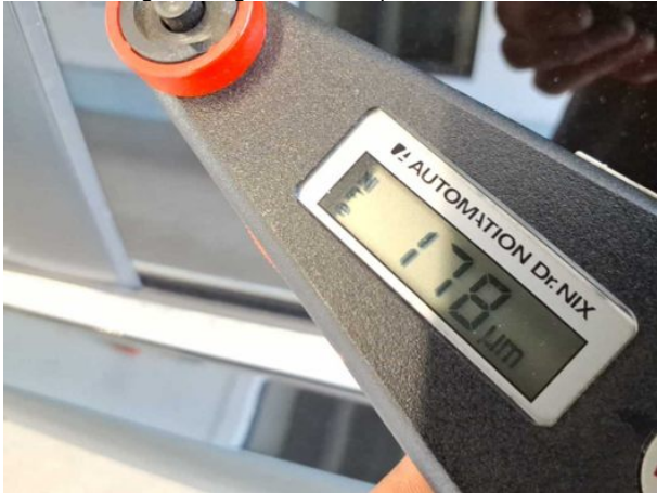
Repainting 1: Roof rail - left side, Roof rail - right side, Mudguard - left side, Mudguard - right side, Side panel - rear left side, Door -
