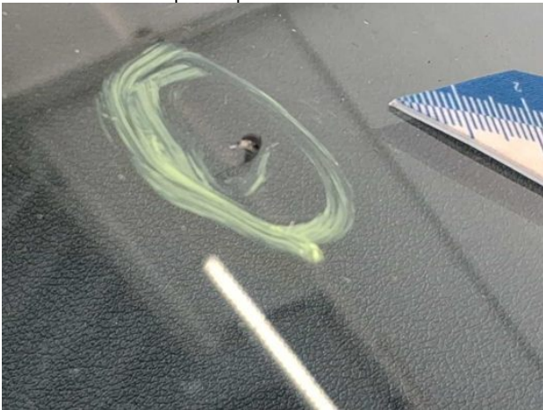
Damage #5: Vehicle glazing: Windscreen with lane departure assistant - Stone chips - Replace
