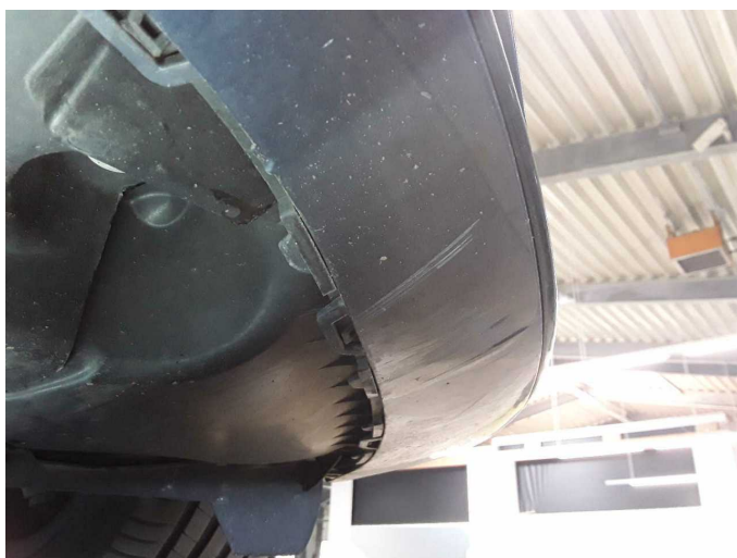
Damage 5: Front bumper: Front bumper - Scratch(es) - Paint
