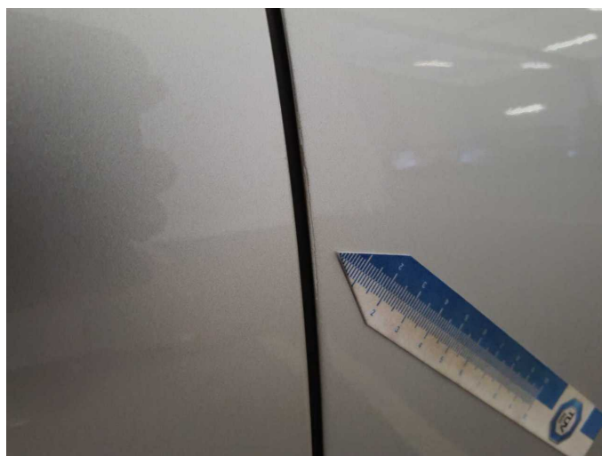
Damage 7: Door - front right side: Door edge - Scratch(es) - Smart repair
