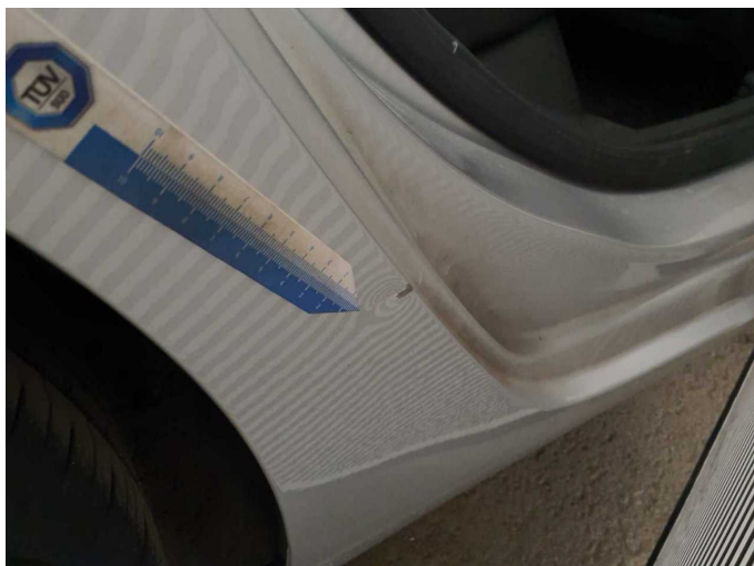
Damage 9: Side panel - rear right side: Elbow - Dent / paintcoat damage - Repair and paint
