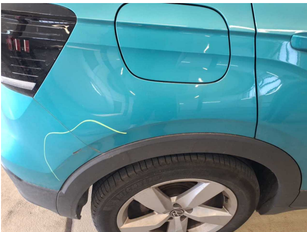
Damage #6: Side panel - rear right side: Side panel - Scratched - Smart repair
