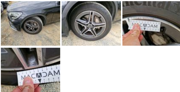
Wing FL, Dent(s), Repair and paint (complete)
