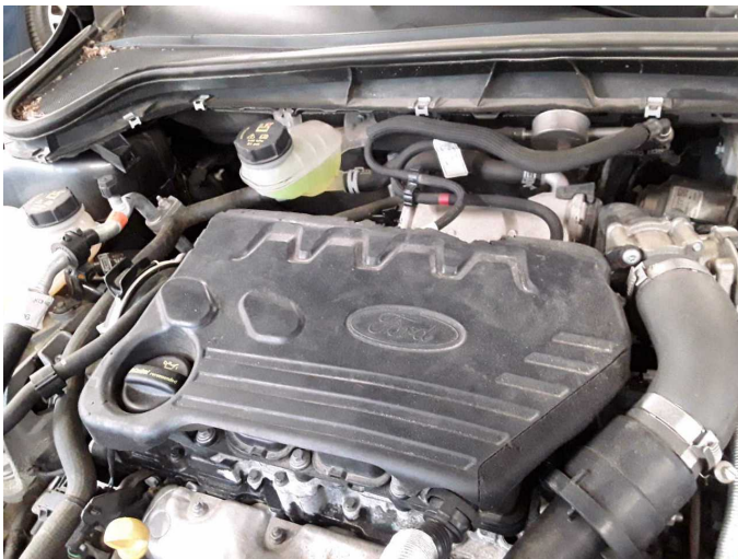
Damage 2: Engine: Engine cover - Damaged - Replace
