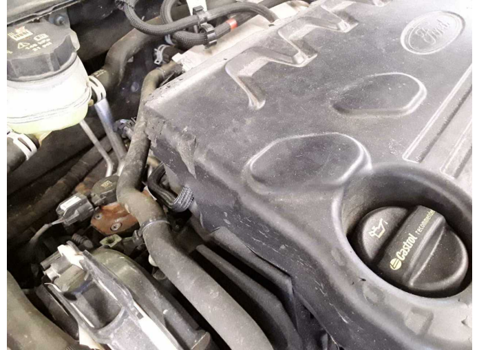
Damage 2: Engine: Engine cover - Damaged - Replace
