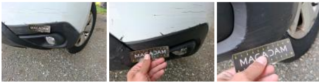
Bumper moulding FL, Scratch(es), Replace
