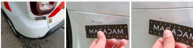
Bumper moulding RL, Broken, Replace
