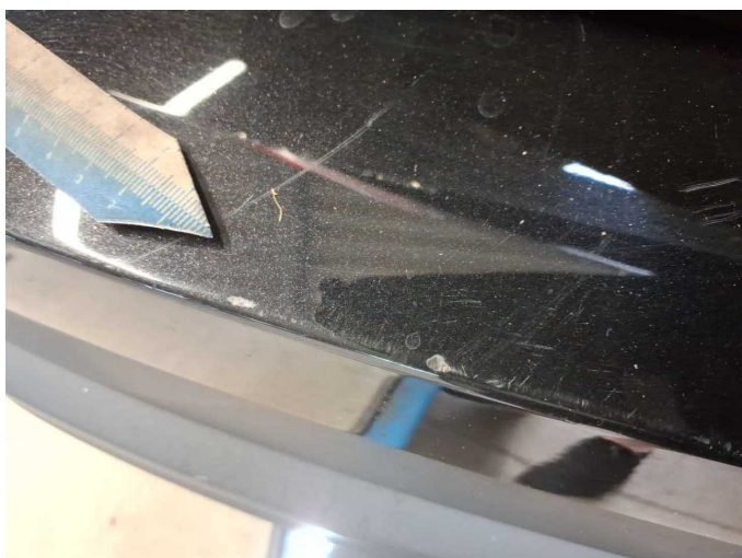
Damage 6: Rear bumper: Rear bumper - Scratched - Paint
