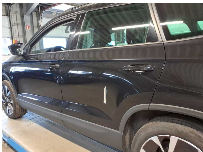
Damage 7: Door - rear left side: Door - Scratch(es) - Paint
