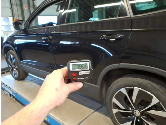
Repainting 7: Door - rear left side
