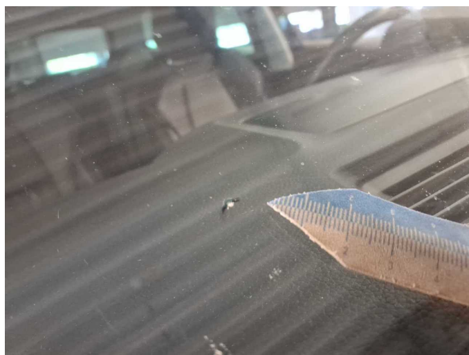
Damage 9: Vehicle glazing: Windscreen - Stone chips - Replace
