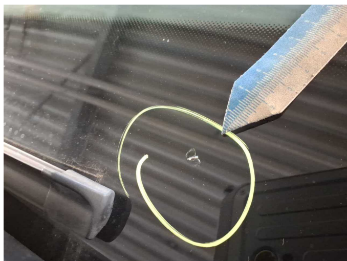
Damage 9: Vehicle glazing: Windscreen - Stone chips - Replace
