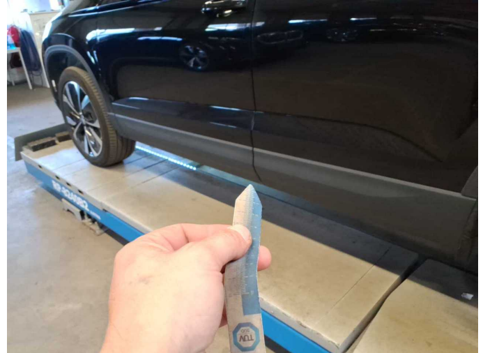
Damage 3: Door - front left side: Brightware - lower - Scratched - Smart repair
