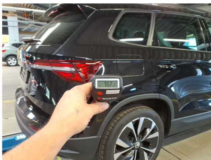
Repainting 6: Side panel - rear right side
