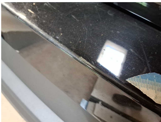
Damage 6: Rear bumper: Rear bumper - Scratched - Paint
