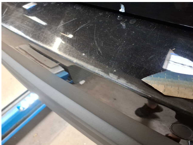
Damage 6: Rear bumper: Rear bumper - Scratched - Paint
