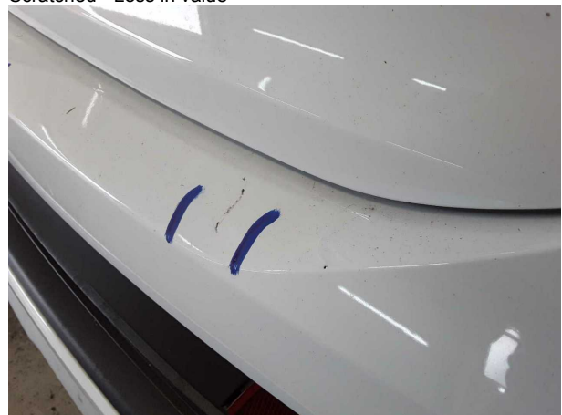
Damage #7: Rear bumper: Rear bumper - Scratched - Smart repair
