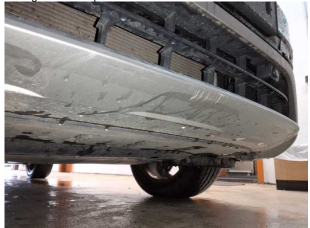
Damage #9: Front bumper: Spoiler - Scratched - Loss in value
