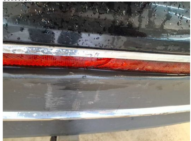
Damage #5: Boot lid / rear door: Reflectors - Damaged - Replace
