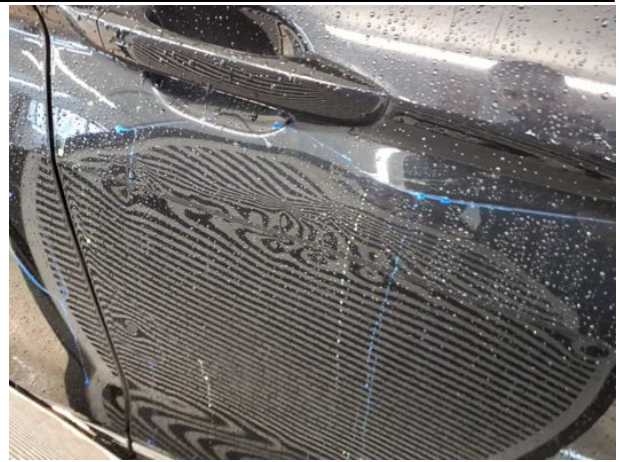
Damage #18: Door - front right side: Door - Dent / paintcoat damage - Repair and paint
