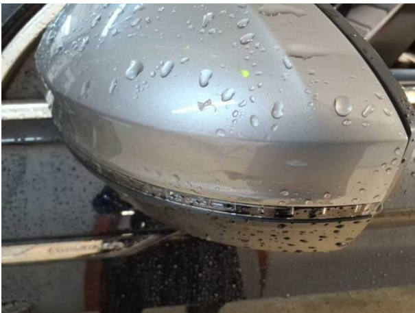
Damage #3: Wing mirror - left side: Cap - Abrasion - Cover / polish
