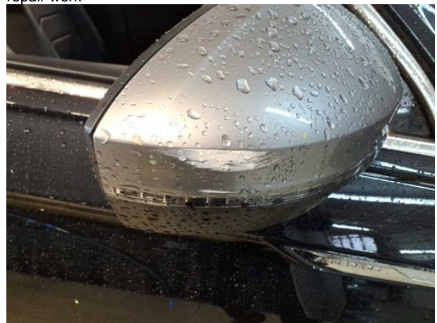
Damage #13: Wing mirror - right side: Cap - Scratched - Replace
