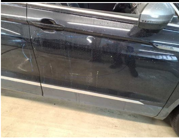
Damage #18: Door - front right side: Door - Dent / paintcoat damage - Repair and paint
