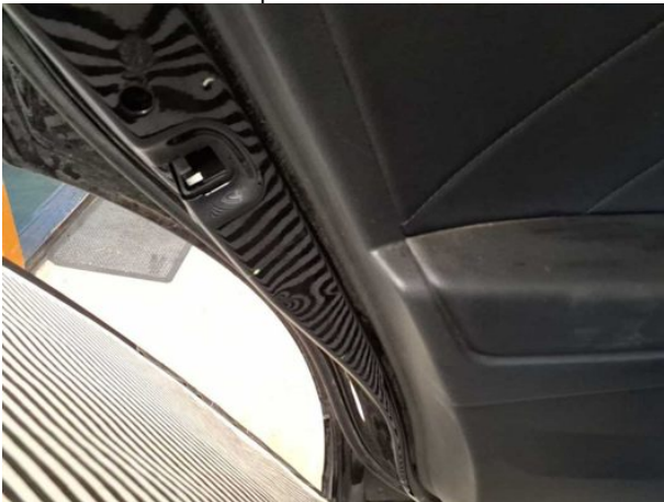
Beschädigung #8: Tür hinten links: Tür - Delle / Lackschaden - Smart Repair
