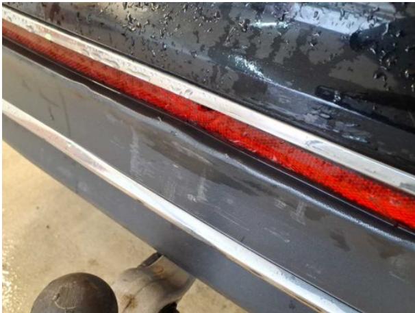
Damage #15: Rear bumper: Spoiler - Deformed - Replace
