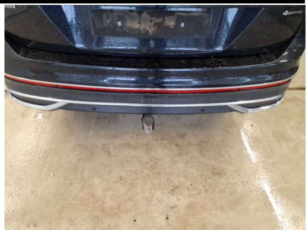
Damage #15: Rear bumper: Spoiler - Deformed - Replace
