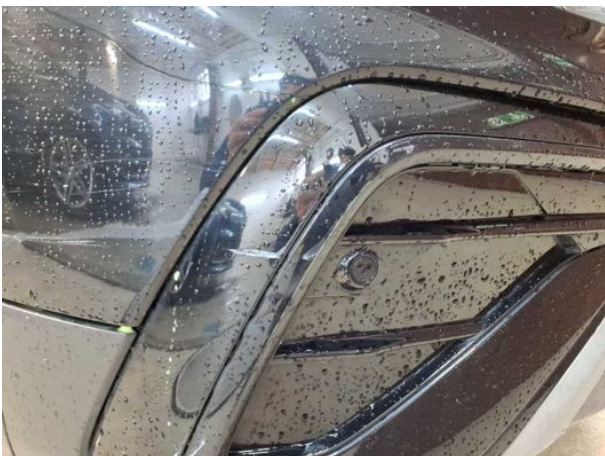
Damage #6: Front bumper: Air-inlet grille - Damaged - Replace
