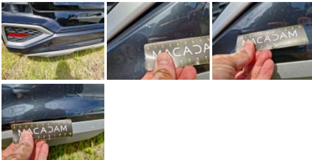
Bumper moulding R, Deformed / Strained, Replace and paint
