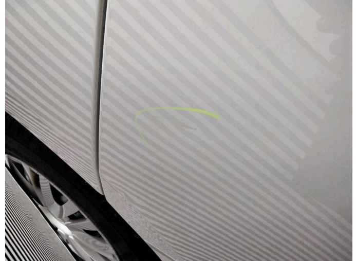
Damage 2: Sliding door, right: Sliding door - Dent / paintcoat damage - Repair and paint
