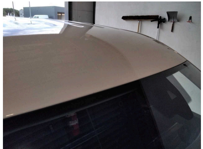
Damage 3: Roof: Roof - dent(s) - Repair and paint
