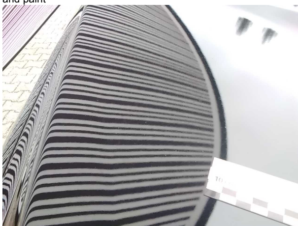
Damage 6: Bonnet: Bonnet - Unprofessionally repaired - Repair and paint
