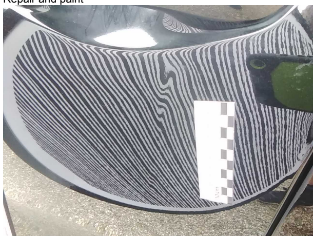
Damage 10: Door - front left side: Door - dent(s) - Repair and paint
