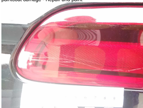
Damage 8: Tail light: Tail lamp - left side - Scratch(es) - Replace
