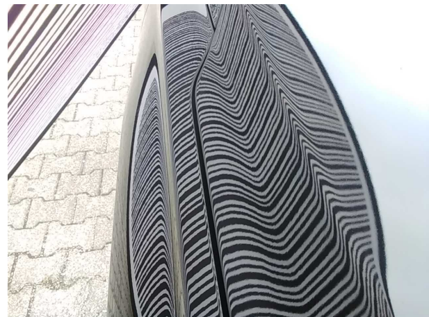
Damage 6: Bonnet: Bonnet - Unprofessionally repaired - Repair and paint
