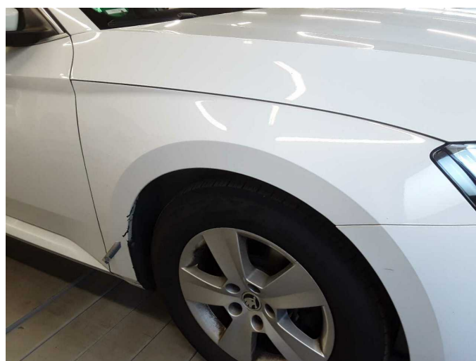
Damage 2: Mudguard - right side: Mudguard - right side - Paint defect - Smart repair
