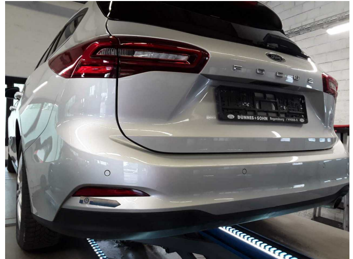
Damage 6: Rear bumper: Rear bumper - Deformed - Repair and paint
