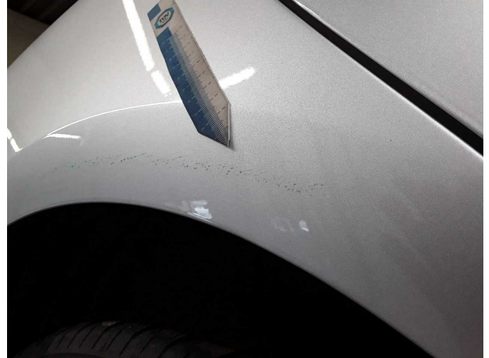
Damage 7: Side panel - rear right side: Side panel (Farbe) - Paint defect - Paint
