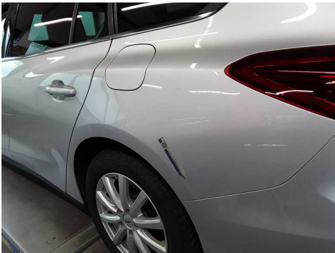
Wear and tear 1: Side panel - rear left side: Side panel - Scratch(es) - No deduction
