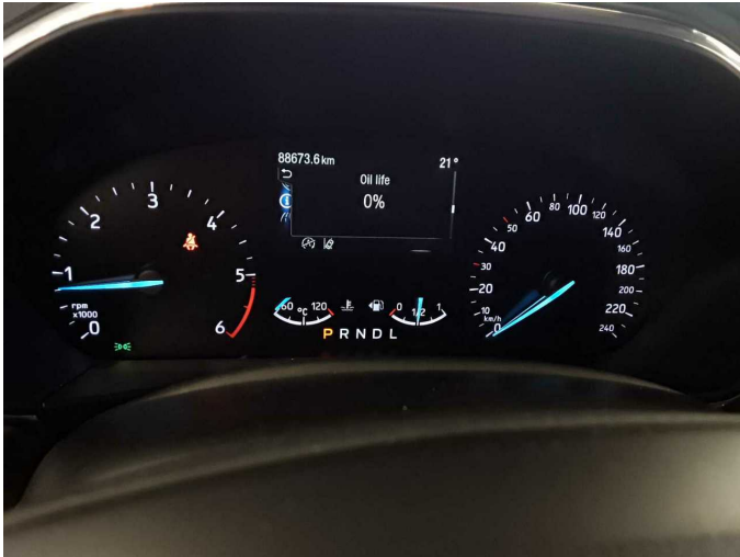
Damage 5: Misc.: Inspection / maintenance - Due - Perform
