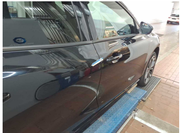
Damage 6: Door - rear right side: Door - Scratch(es) - Smart repair
