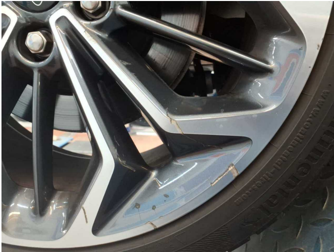
Damage 7: Wheel / tyres: Alloy rim - rear right side - Scratch(es) - Loss in value
