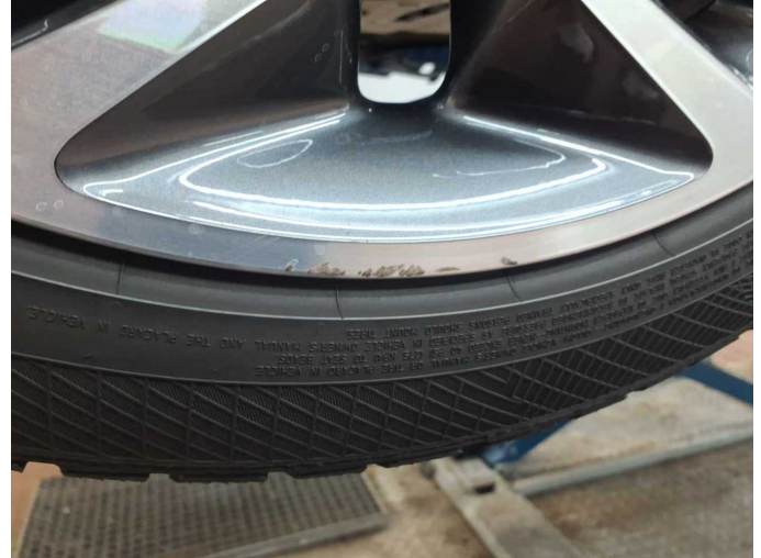
Damage 4: Wheel / tyres: Alloy rim - front left side - Scratch(es) - Loss in value
