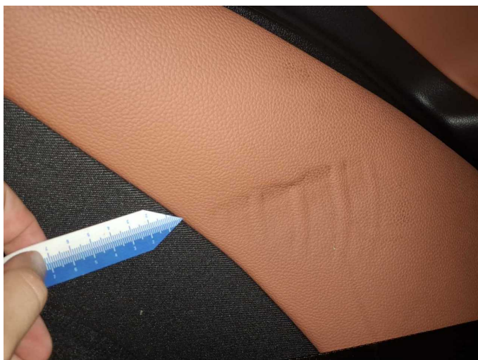
Damage 3: Side panel - rear left side: Interior trim (Polster Einstieg Links; Reifenabdruck) - Smart repair
