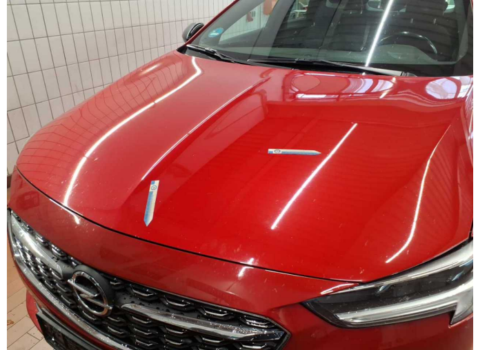
Damage 15: Bonnet: Bonnet - Stone chips - Paint
