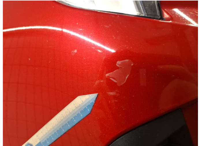
Damage 12: Front bumper: Front bumper - Paint defect - Paint
