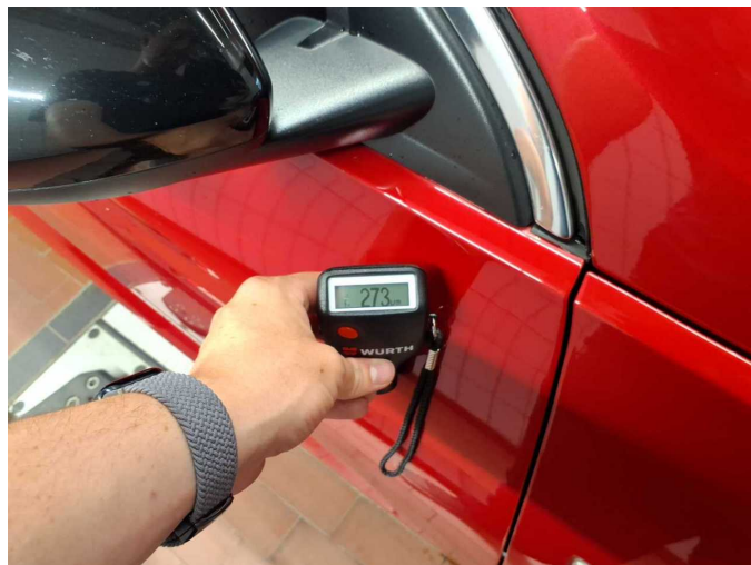
Repainting 6: Door - front right side
