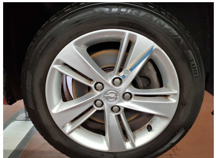
Wear and tear 1: Wheel / tyres: Alloy rim - front right side - Scratch(es) - No deduction
