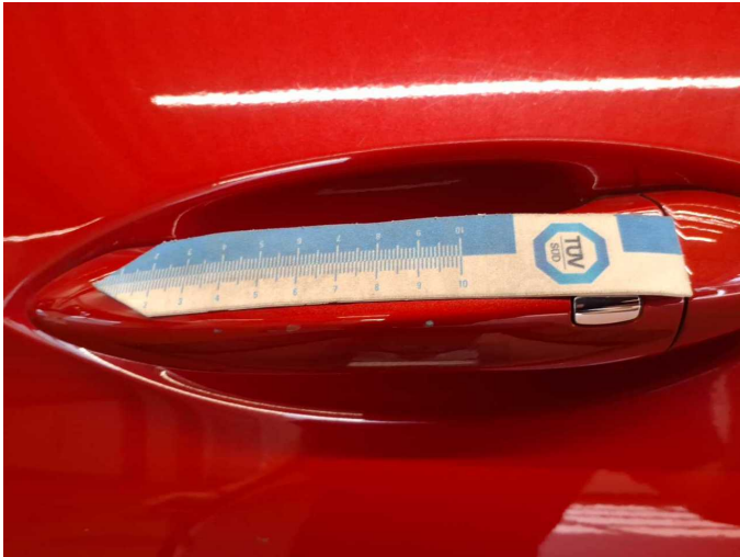
Damage 2: Door - front left side: Door handle - outside - Scratch(es) - Smart repair
