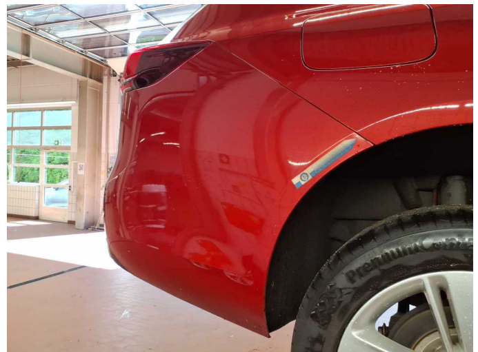
Damage 13: Rear bumper: Rear bumper - Unprofessionally repaired - Repair and paint
