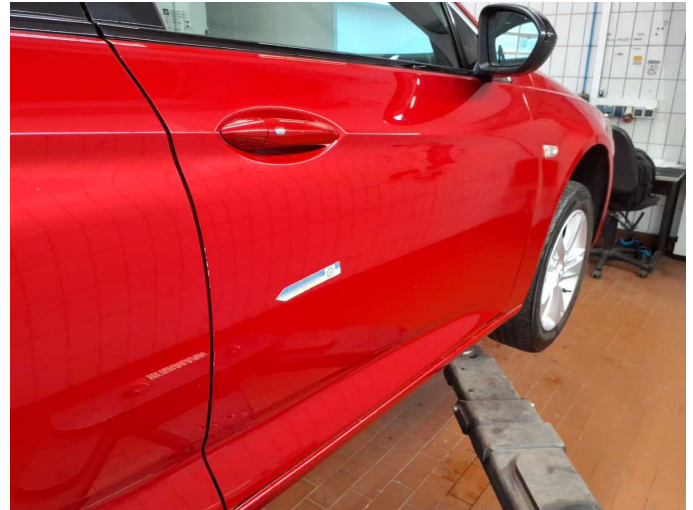
Damage 5: Door - front right side: Door - dent(s) - Smooth repair work
