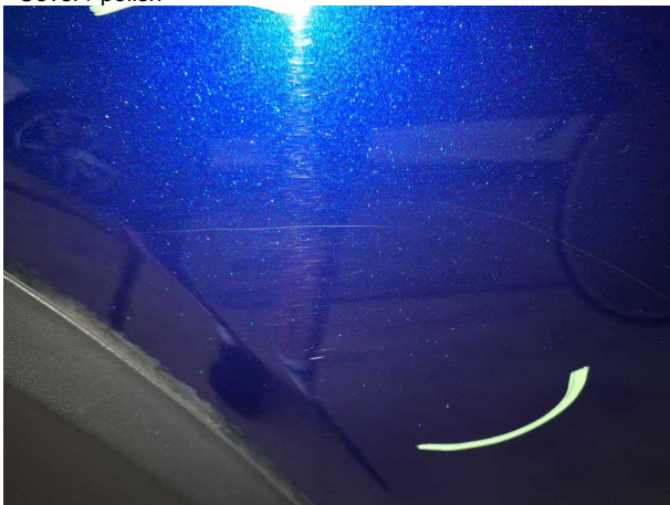
Damage #2: Door - rear right side: Door - Dent / paintcoat damage - Cover / polish
