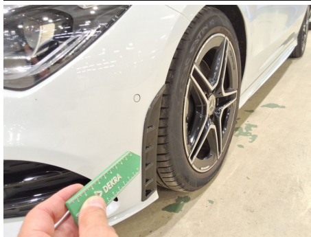
Bumper deflector / Front Left / Non Compliant
