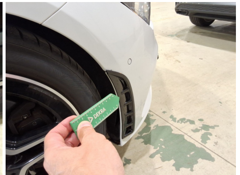
Bumper deflector / Front Right / Non Compliant
