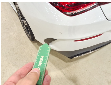
Bumper deflector / Back / Non Compliant
