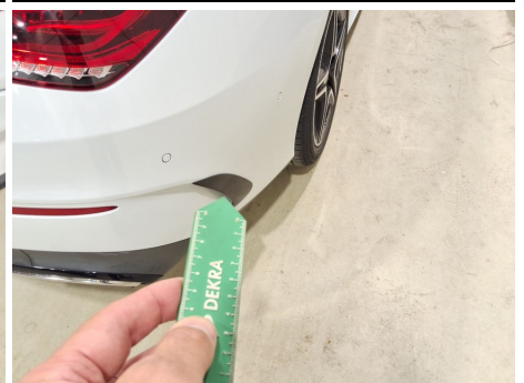
Bumper deflector / Back / Non Compliant
