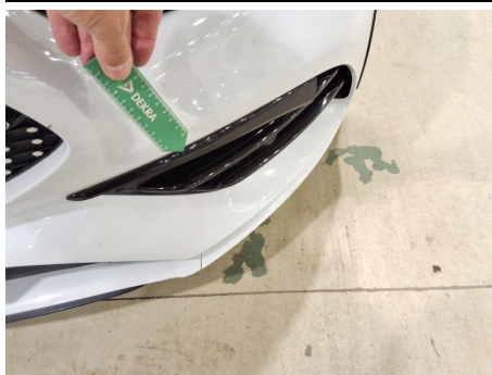
Bumper moulding / Front / Non Compliant
