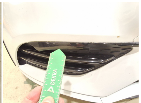
Bumper moulding / Front / Non Compliant
