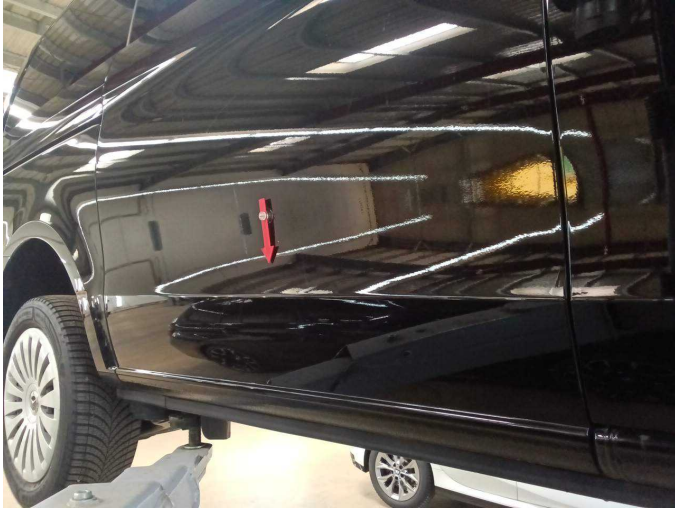
Damage 7: Sliding door, right: Sliding door - Scratched - Paint
