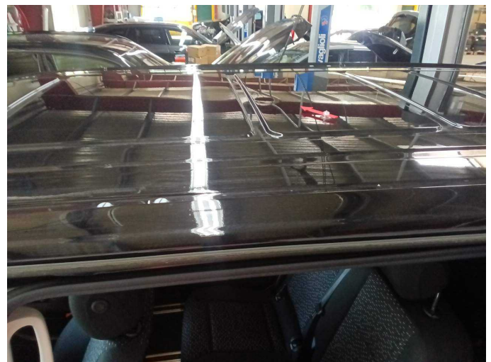
Damage 2: Roof: Roof - dent(s) - Smooth repair work
