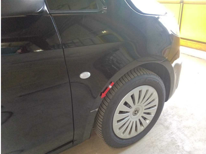
Damage 5: Mudguard - right side: Mudguard - right side - Dent / paintcoat damage - Repair and paint
