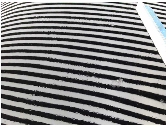
Damage 3: Bonnet: Bonnet (Schleifspuren) - Unprofessionally repaired - Paint
