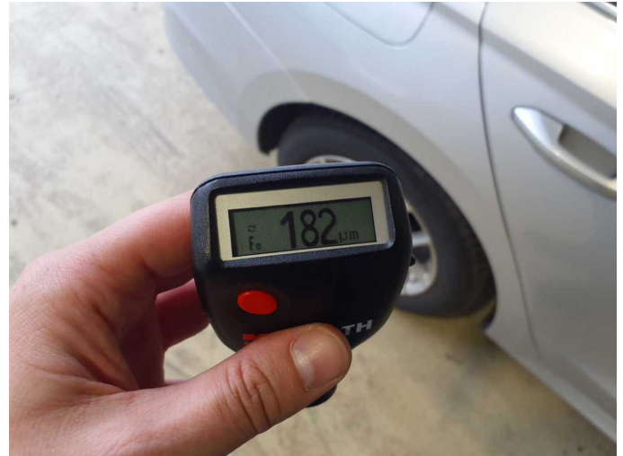
Repainting 3: Side panel - rear right side
