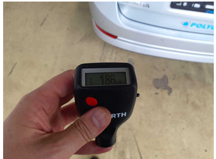
Repainting 1: Boot lid / rear door
