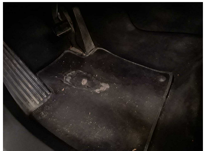
Damage 1: Trim / covers: Floor mats - Damaged - Replace
