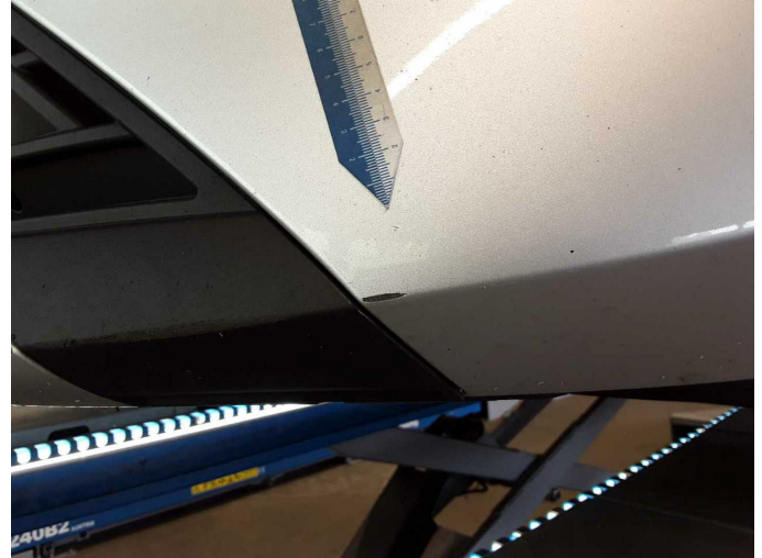
Damage 4: Front bumper: Front bumper - Scratch(es) - Paint
