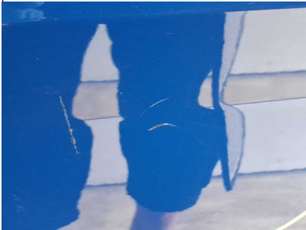
Damage #12: Door - rear left side: Door - Scratched - Repair and paint
