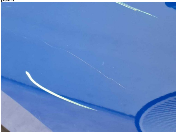
Damage #13: Side panel - rear left side: Side panel - Scratch(es) - Repair and paint
