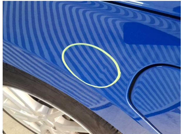
Damage #7: Mudguard - left side: Mudguard - left side - dent(...) - Smooth repair work
