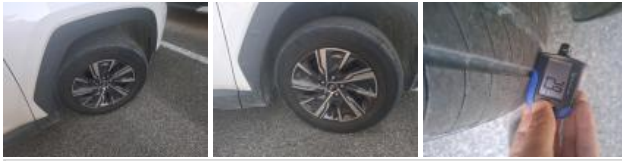
Tyre RR, Out of tolerance, Replace
