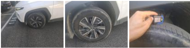
Tyre RL, Out of tolerance, Replace
