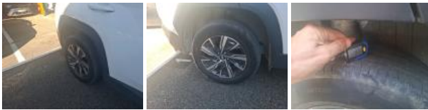
Tyre FL, Out of tolerance, Replace
