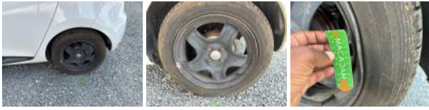
Steel rim RL, Deformed / Strained, Replace
