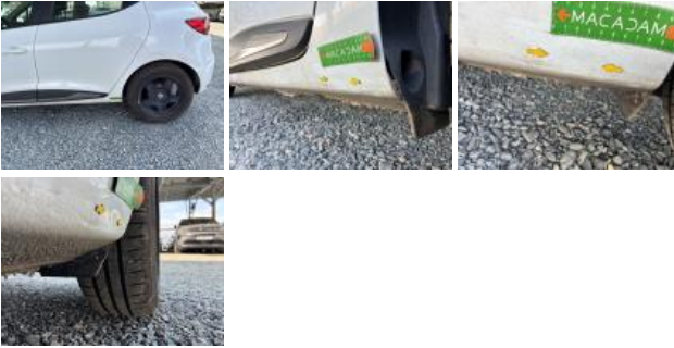
Bumper F, Crack, Replace and paint
