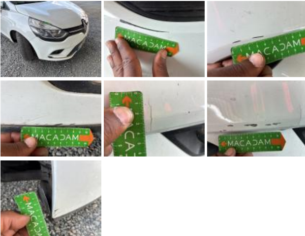
Number plate F, Deformed / Strained, Repair/replace (lump sum)
