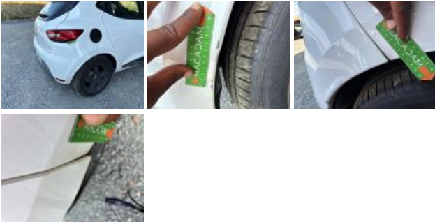
Fuel cap cover, Incomplete, Replace
