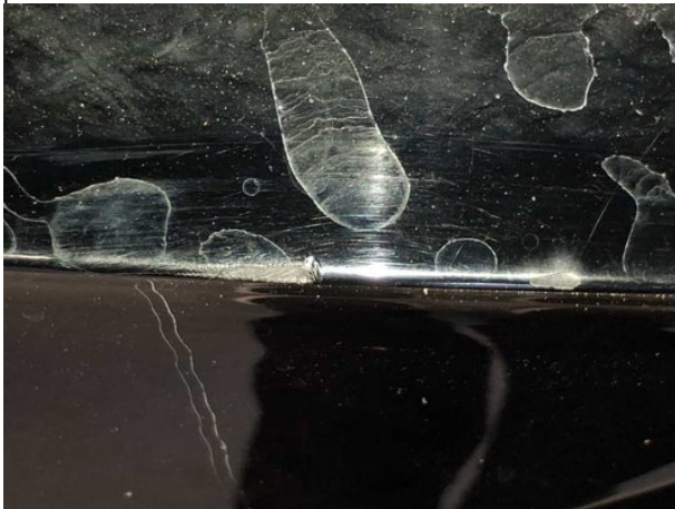
Damage #4: Rear bumper: Rear bumper - Scratch(es) - Repair a... paint
