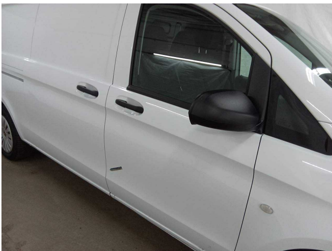
Damage 1: Door - front right side: Door edge - Scratch(es) - Smart repair
