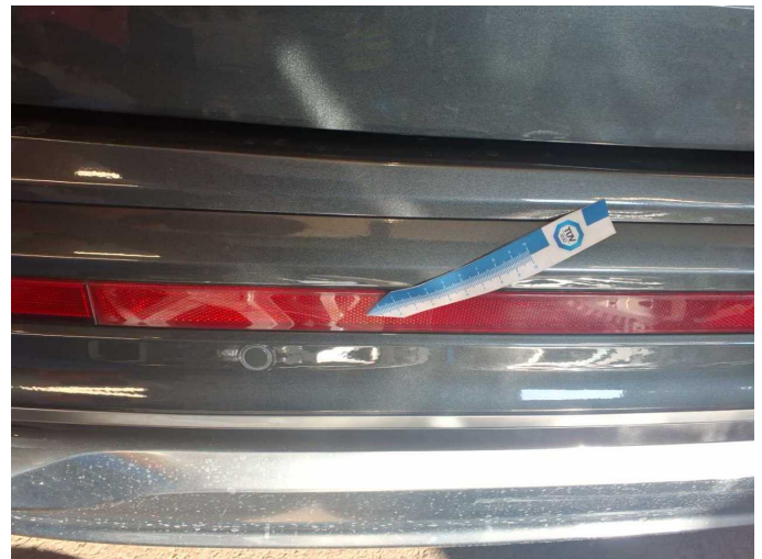
Damage 3: Boot lid / rear door: Reflectors - Scratch(es) - Replace
