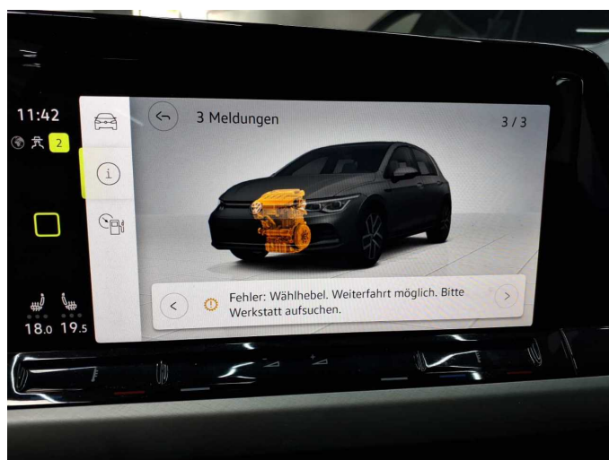
Damage 7: Instrument panel: Indicator light (Getriebe) - on - Perform diagnosis
