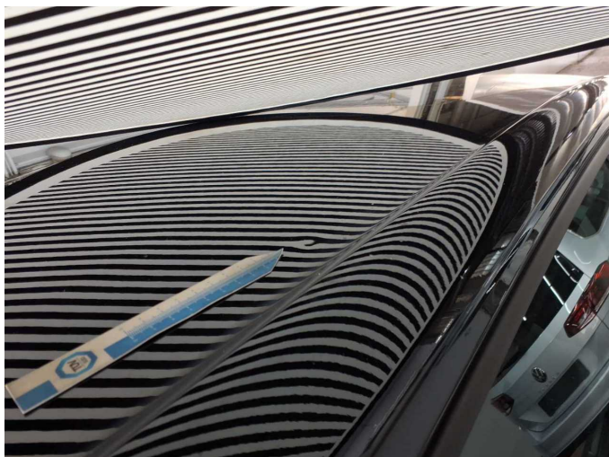
Damage 4: Roof: Roof - dent(s) - Smooth repair work
