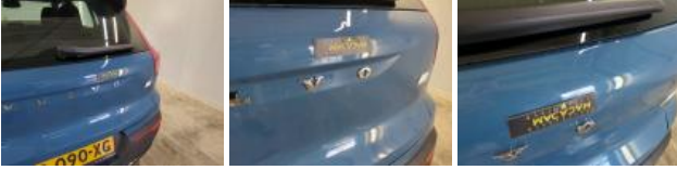
Tailgate / Boot, Dent(s), Repair and paint (complete)
