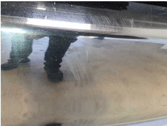
Damage 10: Rear bumper: Rear bumper - Scratch(es) - Paint
