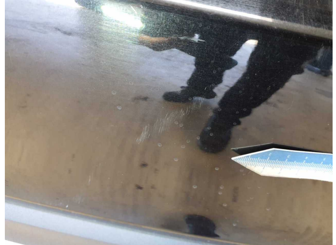
Damage 10: Rear bumper: Rear bumper - Scratch(es) - Paint
