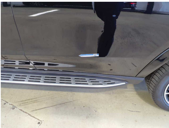
Damage 5: Door - rear left side: Door - dent(s) - Smart repair
