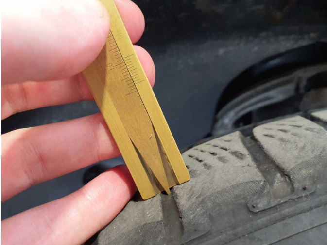
Damage 6: Wheel / tyres: Tyre - front right side - Worn - Replace
