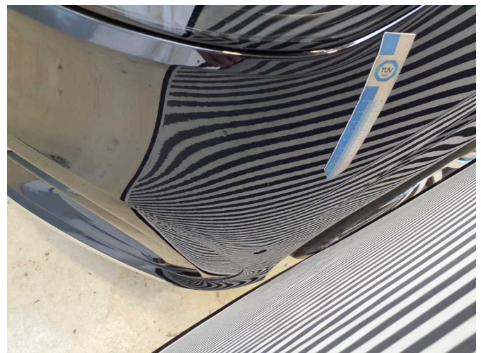
Damage 11: Front bumper: Front bumper (Einschlüsse und orangenhaut) - Unprofessionally repaired - Repair and paint
