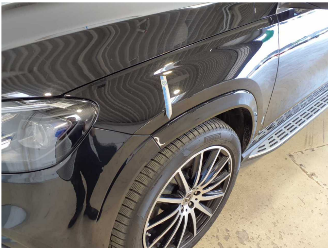
Damage 4: Mudguard - left side: Wheel well extension (Orangenhaut) - Paint defect - Repair and paint
