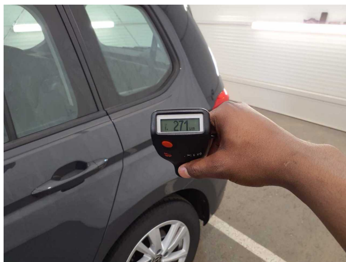
Repainting 1: Side panel - rear left side
