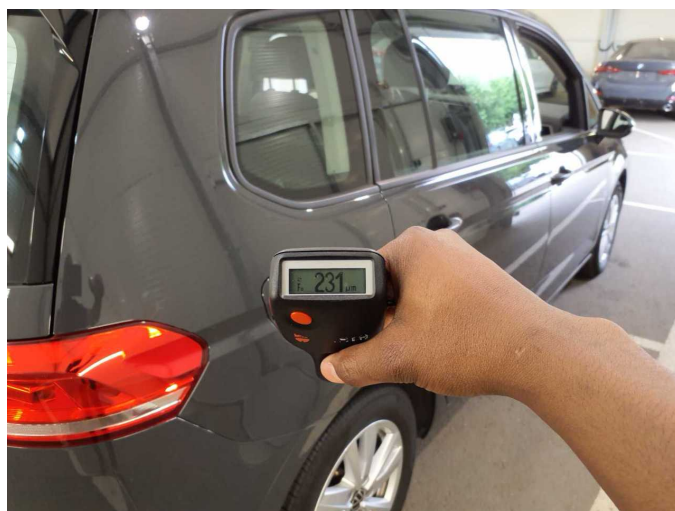
Repainting 2: Side panel - rear right side
