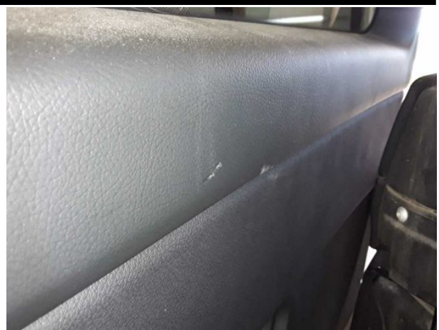
Damage #4: Trim / covers: Door trim - rear right side - Damaged - Loss in value
