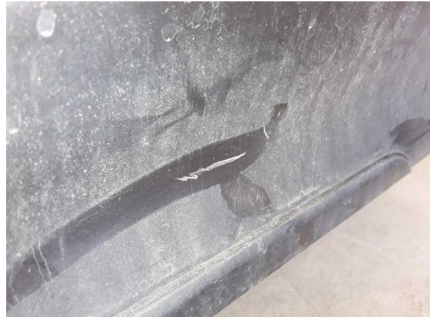
Damage #2: Rear bumper: Rear bumper - Scratched - Loss in value
