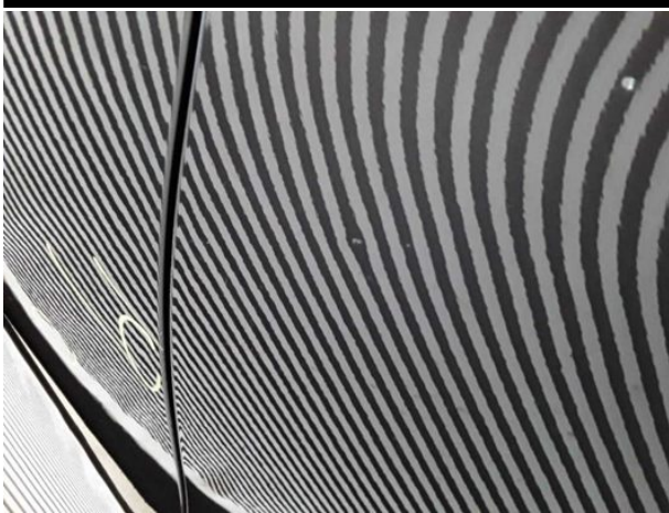
Damage #7: Door - front right side: Door - Dent / paintcoat damage - Smart repair
