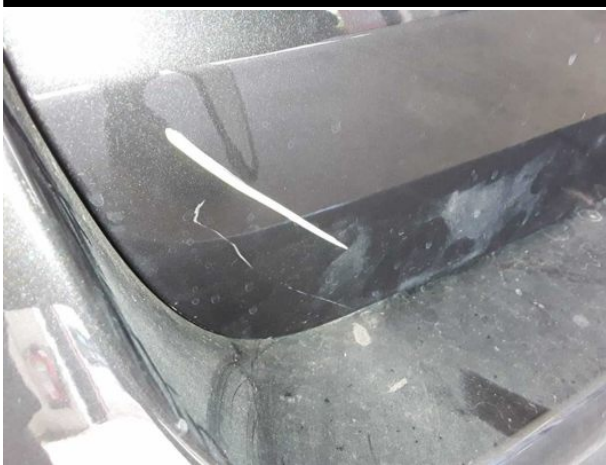
Damage #9: Boot lid / rear door: Boot lid - Scratched - Smart repair
