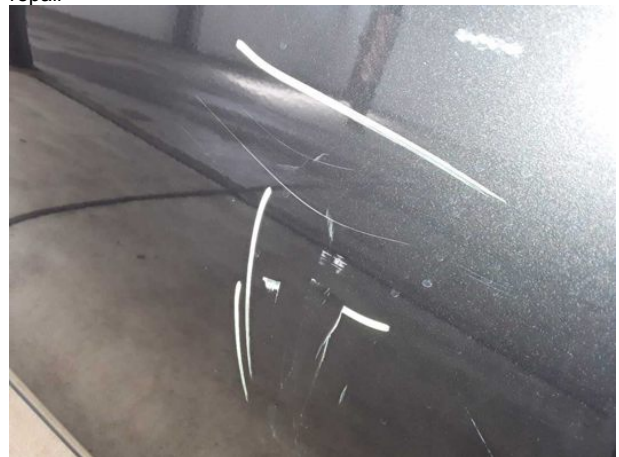
Damage #10: Sliding door, right: Sliding door with glass panel - Dent / paintcoat damage - Repair and paint
