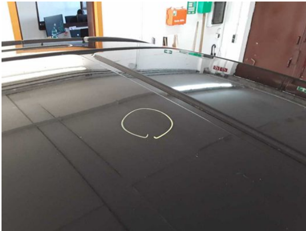
Damage #5: Roof: Roof - dent(s) - Smooth repair work
