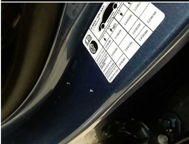
Damage #5: Sill - left side: Sill - Dent / paintcoat damage - Smart repair
