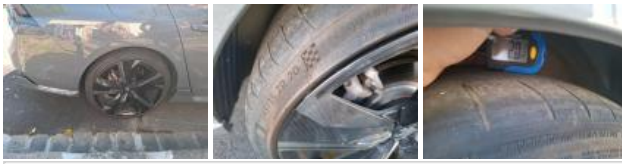
Tyre RL, Out of tolerance, Replace
