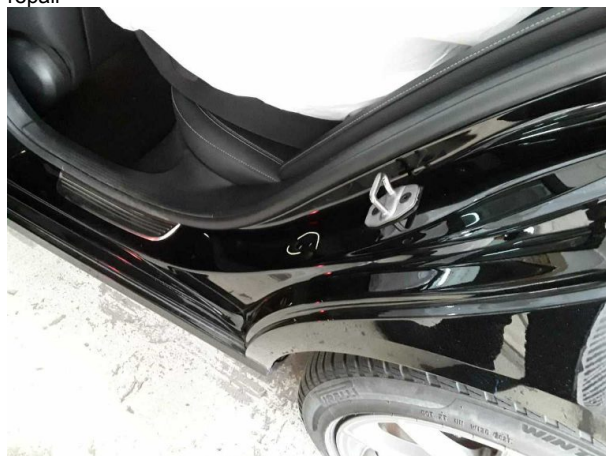
Damage #9: Side panel - rear left side: Sill - Dent / paintcoat damage - Repair and paint
