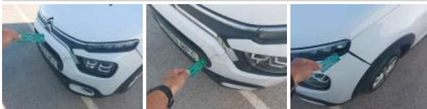
Fog lamp L, Missing, Replace
