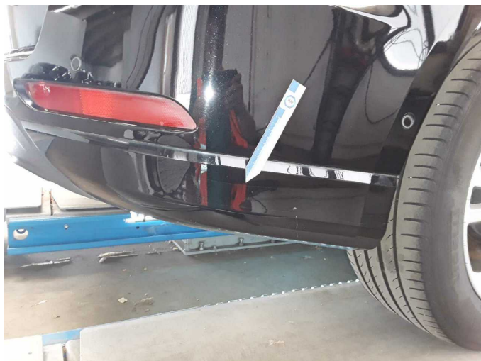
Damage 8: Rear bumper: Rear bumper - Scratch(es) - Paint
