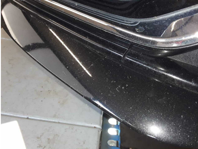
Damage 11: Front bumper: Front bumper - Stone chips - Paint
