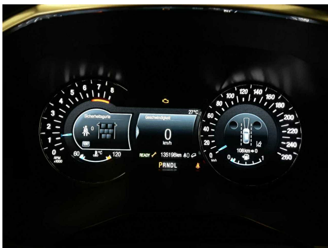
Damage 7: Instrument panel: Indicator light (Motorkontrollleuchte) - on - Perform diagnosis
