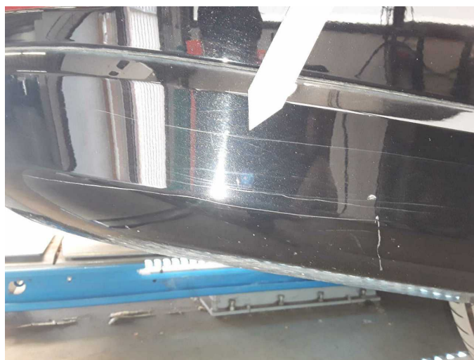
Damage 8: Rear bumper: Rear bumper - Scratch(es) - Paint
