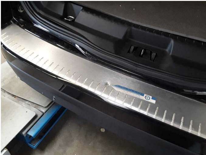
Damage 2: Rear bumper: Cover - bumper - rear - Damaged - Replace
