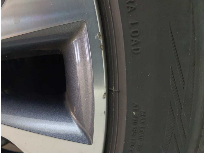
Damage 4: Wheel / tyres: Alloy rim - rear right side - Scratched - Loss in value
