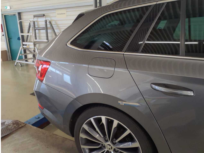
Damage 2: Side panel - rear right side: Side panel - dent(s) - Smart repair
