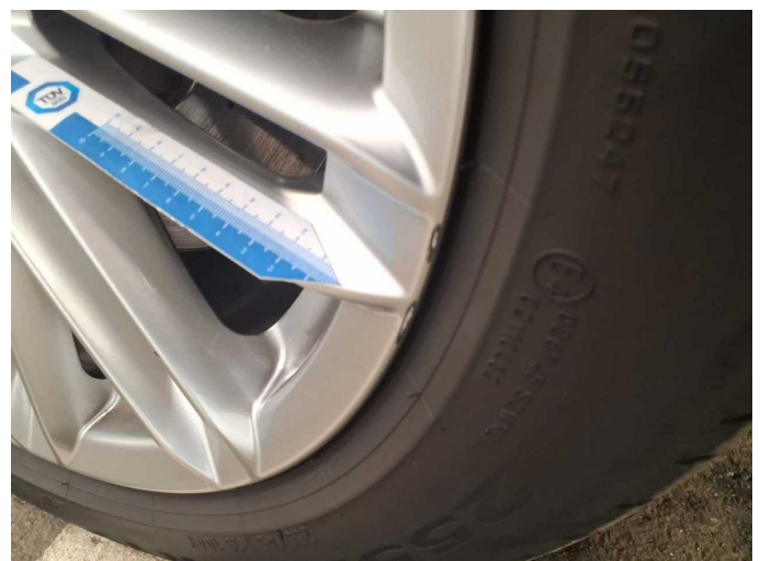
Damage 3: Wheel / tyres: Alloy rim - front right side - Scratched - Loss in value
