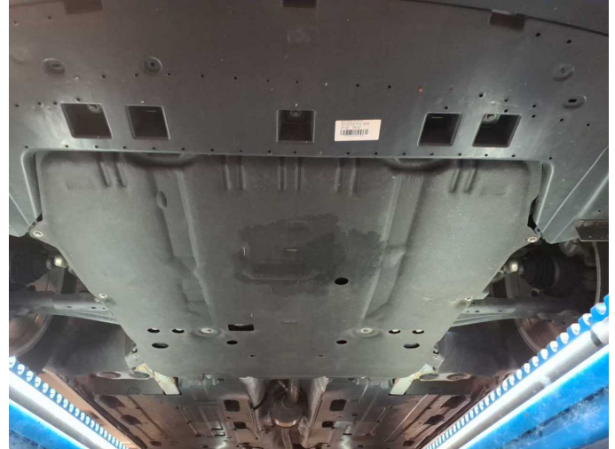
Damage 4: Engine: Engine (Motor/Getriebe) - Leaking - Perform diagnosis
