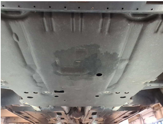
Damage 4: Engine: Engine (Motor/Getriebe) - Leaking - Perform diagnosis
