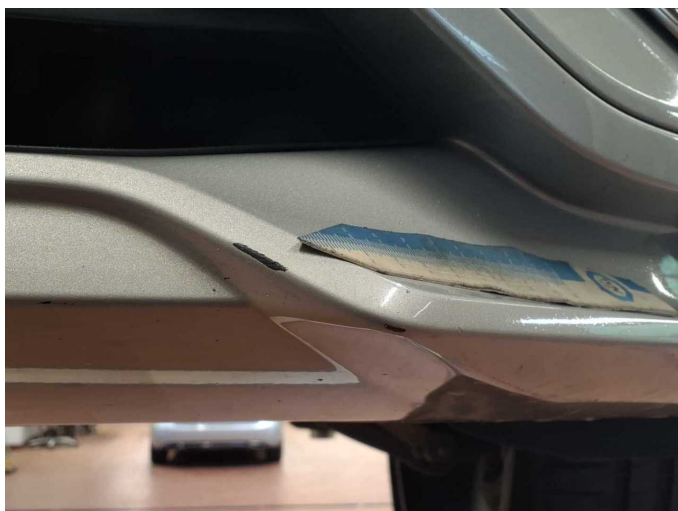
Damage 13: Front bumper: Spoiler - Scratched - Paint
