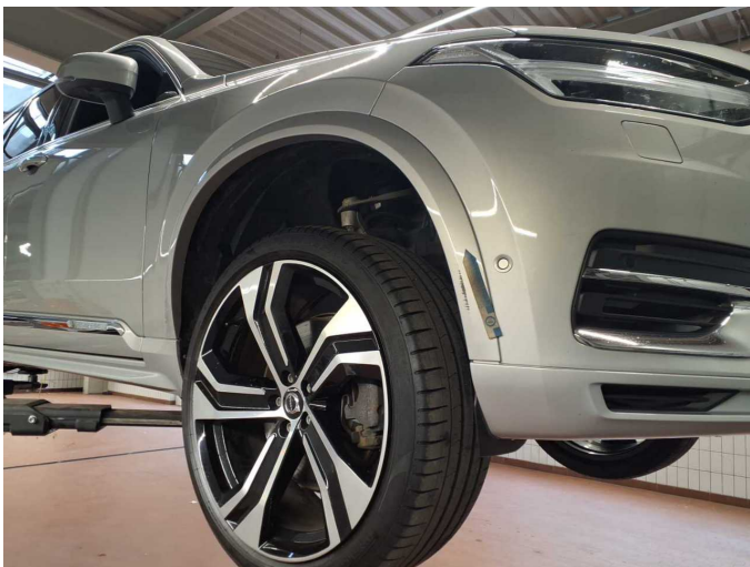
Damage 11: Mudguard - right side: Wheel well extension - Scratched - Paint
