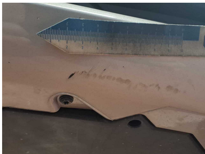
Damage 13: Front bumper: Spoiler - Scratched - Paint
