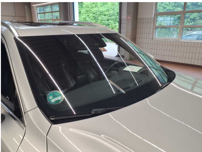
Damage 15: Vehicle glazing: Windscreen - Stone chips - Replace
