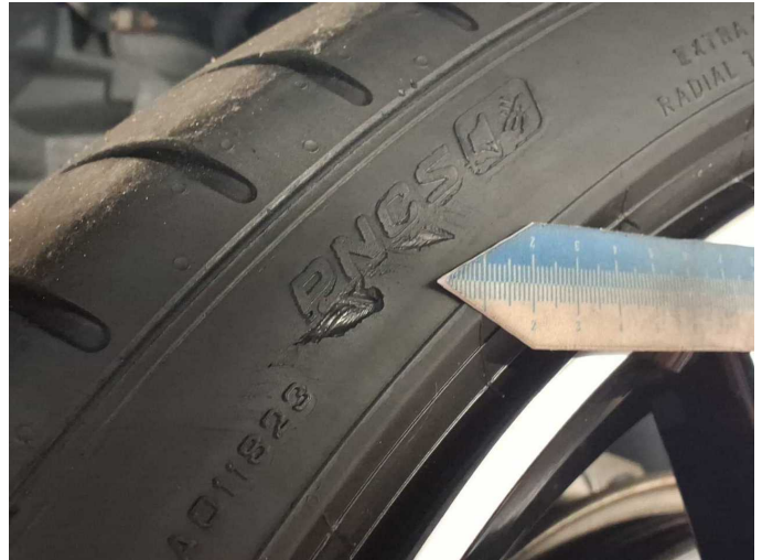
Damage 10: Wheel / tyres: Tyre - front right side - Broken / torn - Replace
