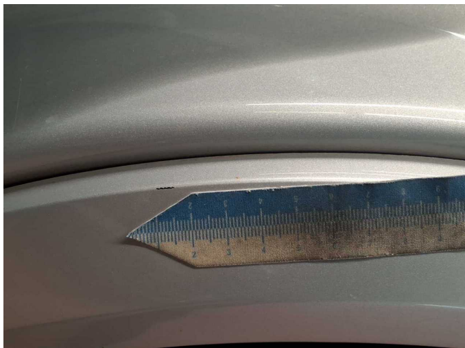
Damage 12: Side panel - rear left side: Wheel well extension - Scratched - Paint
