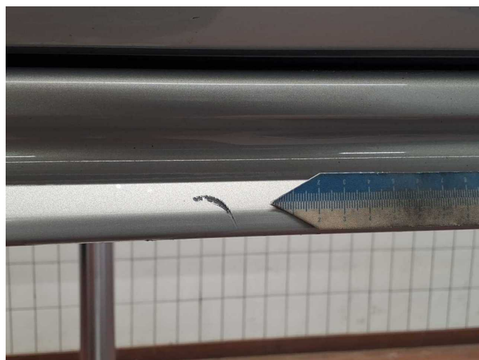
Damage 5: Sill - left side: Trim - Scratch(es) - Smart repair
