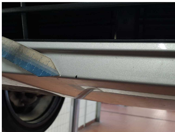
Damage 13: Front bumper: Spoiler - Scratched - Paint
