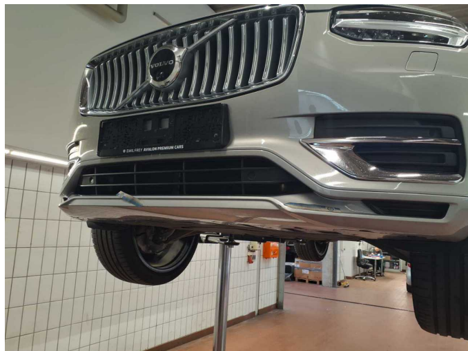
Damage 13: Front bumper: Spoiler - Scratched - Paint
