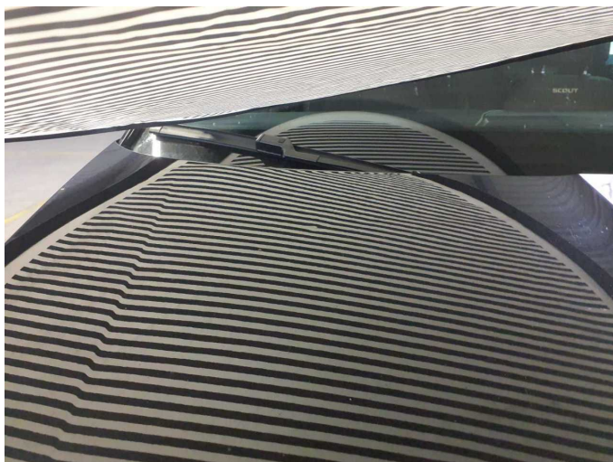
Damage 5: Bonnet: Bonnet - Dent / paintcoat damage - Paint
