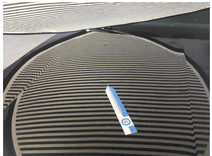
Damage 5: Bonnet: Bonnet - Dent / paintcoat damage - Paint
