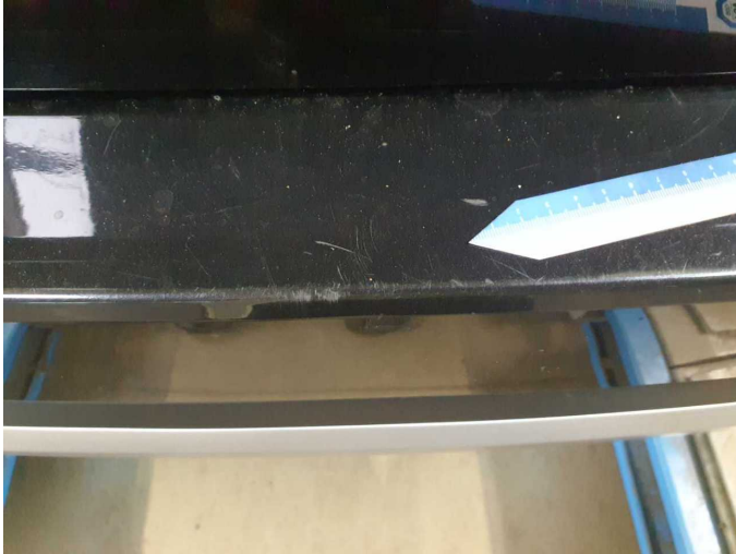
Damage 4: Rear bumper: Rear bumper - Scratched - Paint
