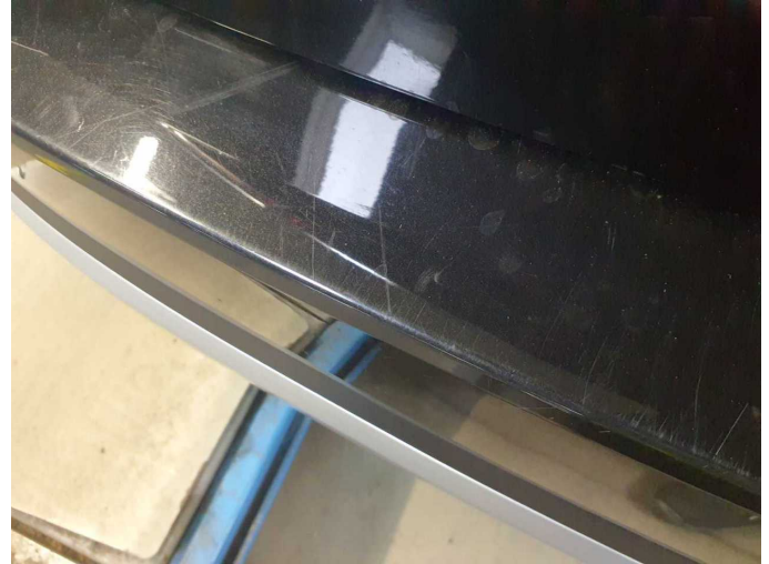
Damage 4: Rear bumper: Rear bumper - Scratched - Paint
